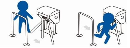
Emergency escape function: Equipped with emergency escape control device, one of the arms will dropdown automatically to evacuate pedestrians conveniently.
