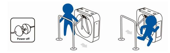
Emergency escape function: Equipped with emergency escape control device, one of the arms will dropdown automatically to evacuate pedestrians conveniently.
