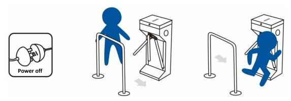
Emergency escape function: Equipped with emergency escape control device, one of the arms will drop automatically to evacuate pedestrians conveniently.
