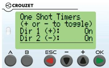
This screen allows for the two one-shot timer settings to be enabled or disabled. This setting prevents access control from holding a direction open on the standard direction inputs. Toggle Direction 1 by pressing + and Direction 2 by pressing -. This should be set to "On" in almost every installation.
