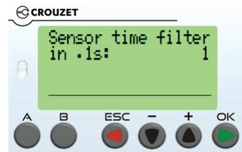
The value on this screen defines how long sensors must be blocked before registering. Lessening the timer will make the units more sensitive. Typically, a range of 1 to 3 is a good setting here. This filters out quick accidental beam crosses without allowing too much through.
