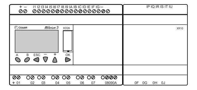
The product needs normally open contact closures between the relevent inputs in order to function. The normally open terminal from a relay would go to the relevant input while the common terminal needs to connect to 24VDC+. Separate inputs for each direction as well as access control vs. hold open are available to allow a variety of different functions depending on the need at the installation.
