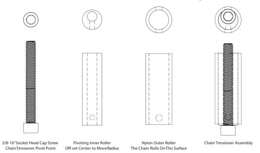
By loosening the socket head cap screw and aligning the side holes on the inner and outer roller with a screwdriver or similarly sized tool, it is possible to change the location of the rollers in relation to the chain, effectively providing a way to adjust the chain's tension.
