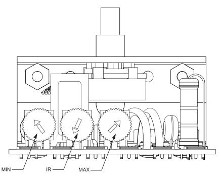
Figure 4 - Control Trimpot Adjustment Location
