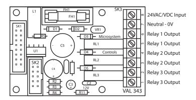
The coin mechanism can be configured to give different outputs in different circumstances, but for the purposes of connecting to a turnstile or gate, only Relay 1 is used. Interfacing the VAL 343 to the turnstile's logic controller is fairly basic. 3 wires are ran from the VAL 343 to the 6500 Series Control Head. This device should be wired as an access control device per the wiring diagram. Specifically, the device connects as follows:
