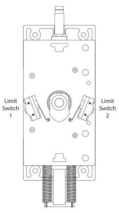
Turnstile control heads use a triangular shaped limit switch cam. One point of the triangle needs to be facing the index pin (bar with two springs) when the cam is in the home position. The two indents in the sides of the triangle are for jigging purposes. It does not matter which point is facing to the springs.
