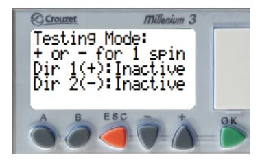
Testing mode simulates valid access control inputs based on the settings defined on the other menu screens. The unit should unlock for the duration of the directional timer or until the unit is rotated. If the button is pressed twice, it should allow two rotations or time out based on the mult-swipe setting. If the button is held and the one shot timers are disabled, the unit will continue to remain open until the button is released and another rotation or timeout occurs.
