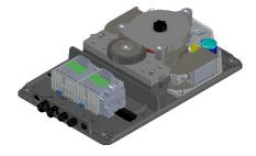
Modern Modular locking mechanism can be configured fail safe or fail secure as well as clockwise or counterclockwise. Because the locking mechanism is modular it is extremely simple and easy to service when needed. Tested to 1 million cycles with zero maintenance.
