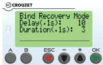
In the event the arm attempts to move forward for the duration of the first value, but is unable due to it being out of position and binding against the locking bar, it will automatically reverse its swing for the second value. The only reason to adjust this is if the motor controller has been set to a reduced speed.
