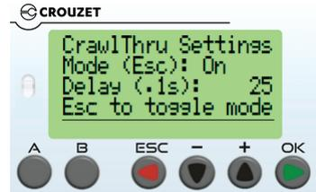
The value on this screen defines how the anti-crawl thru functionality works. If enabled, when sensor S1 is blocked for the adjustable duration shown on this window, the alarm scenario for anti-crawl thru detection is activated. Adjust the timer value by pressing OK then increasing or decreasing the setting and pressing OK again to save. Toggle this setting to disable it or enable it by pressing ESC.
