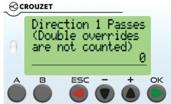
This screen has a readout showing how many people have passed through the lane in direction 1 (outside of a double override scenario). It is good information for maintenance.
