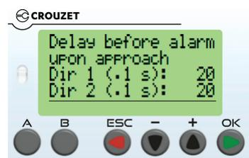
The value is only applicable to controlled passage directions. If the lane is in the home position, the unit will wait for the duration listed before setting the lane into alarm. The reason for this is many times in their haste, people will walk into the lane before swiping their badge. If the arm is open or closing at the time of entry, the alarm will sound regardless of this setting.
