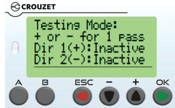
This screen allows for the lane to be activated in either direction based on how the lane is set up. The lane will not activate from this window if a direction is set to free passage. Press + to activate the lane in Direction 1 and - to activate the lane in Direction 2. Multiswipes are also allowed from this window based on the Swipe Queue setting.
