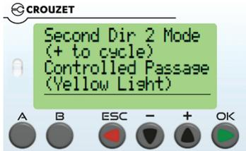
The value on this screen defines the secondary operation of direction 2. Upon applying voltage to the Direction 2 Mode Change input, the lane will switch to this secondary mode of operation. This is handy for facilities that frequently need to change what their lanes are doing. Press + to cycle between Controlled Passage, Free Passage or No Passage.
