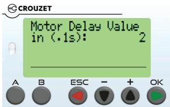
This setting adds a slight pause to the motor before running in the opposite direction to protect the circuitry. There is not really any need to adjust this beyond its preconfigured setting of .2 seconds.
