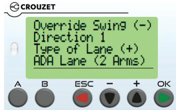
The first setting defines which way the arm swings in the event both directional overrides are activated at the same time. It is toggled between direction 1 and direction 2 by pressing the - Button. The second part is configured in the factory based on the lane type purchased and should not be changed.
