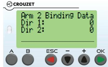
This screen lists how many times the bind recovery scenario happened for either direction on Arm 2. Single arm lanes will automatically skip this window.
