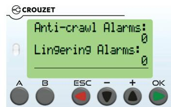
This screen lists how many times the anti-crawl through alarm or the linger in beam alarm occurred (as defined in previous settings).
