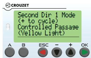
The value on this screen defines the secondary operation of direction 1. Upon applying voltage to the Direction 1 Mode Change input, the lane will switch to this secondary mode of operation. This is handy for facilities that frequently need to change what their lanes are doing. Press + to cycle between Controlled Passage, Free Passage or No Passage.
