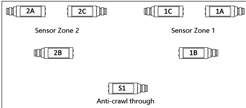
Above is a diagram which illustrates each sensor's position. There are 7 sensors on each cabinet total, separated into 3 "zones".
