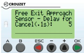
Units purchased as having a free passage direction come with an additional out-facing sensor to activate the lane a bit earlier. While not necessary to operation, it adds to the user friendliness of the lane. This setting adjusts how long it takes for the arm to return if it opened but nobody walked through.
