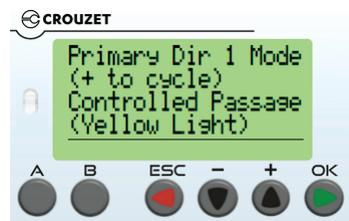
The value on this screen defines the standard operation of direction 1. It can be set to Controlled Passage (w/ yellow indicator lights), Free Passage (w/ green indicator lights) or No Passage (w/ red indicator lights). Controlled or Free are the most common settings, but if there are multiple lanes, using No Passage may help to spread traffic through multiple lanes. This is configured based on our understanding of the job requirements in the factory, but can be cycled by pressing the + button.
