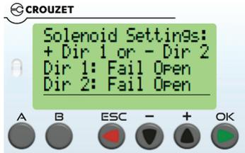
This screen is preconfigured in the factory based on requested operation. Solenoids may be fail open or fail lock in one or both directions. Changing this setting will cause adverse operation unless the appropriate mechanical changes are made to go along with them.
