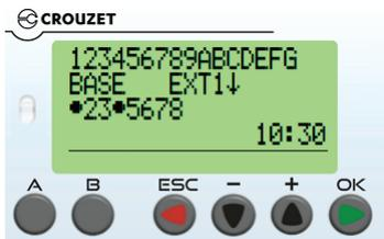
A variety of different readouts and menus for the backend of the logic controller are available. It is best to avoid tinkering here to avoid accidentally resetting the logic and losing all of the project settings. Avoid holding escape and if this manages to enter any further menus, try not to "stop" and then "reset all values and start" the logic.
