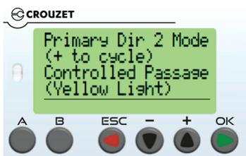
The value on this screen defines the standard operation of direction 2. It works the same as the direction 1 setting. Press + to cycle between Controlled Passage, Free Passage or No Passage.
