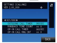
Settings screen (001/008) is displayed. During configuration, the setting indicator is ON.
