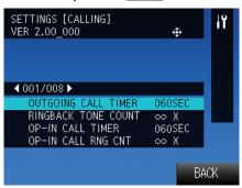
Settings screen (001/008) is displayed. During configuration, the setting indicator is ON.
