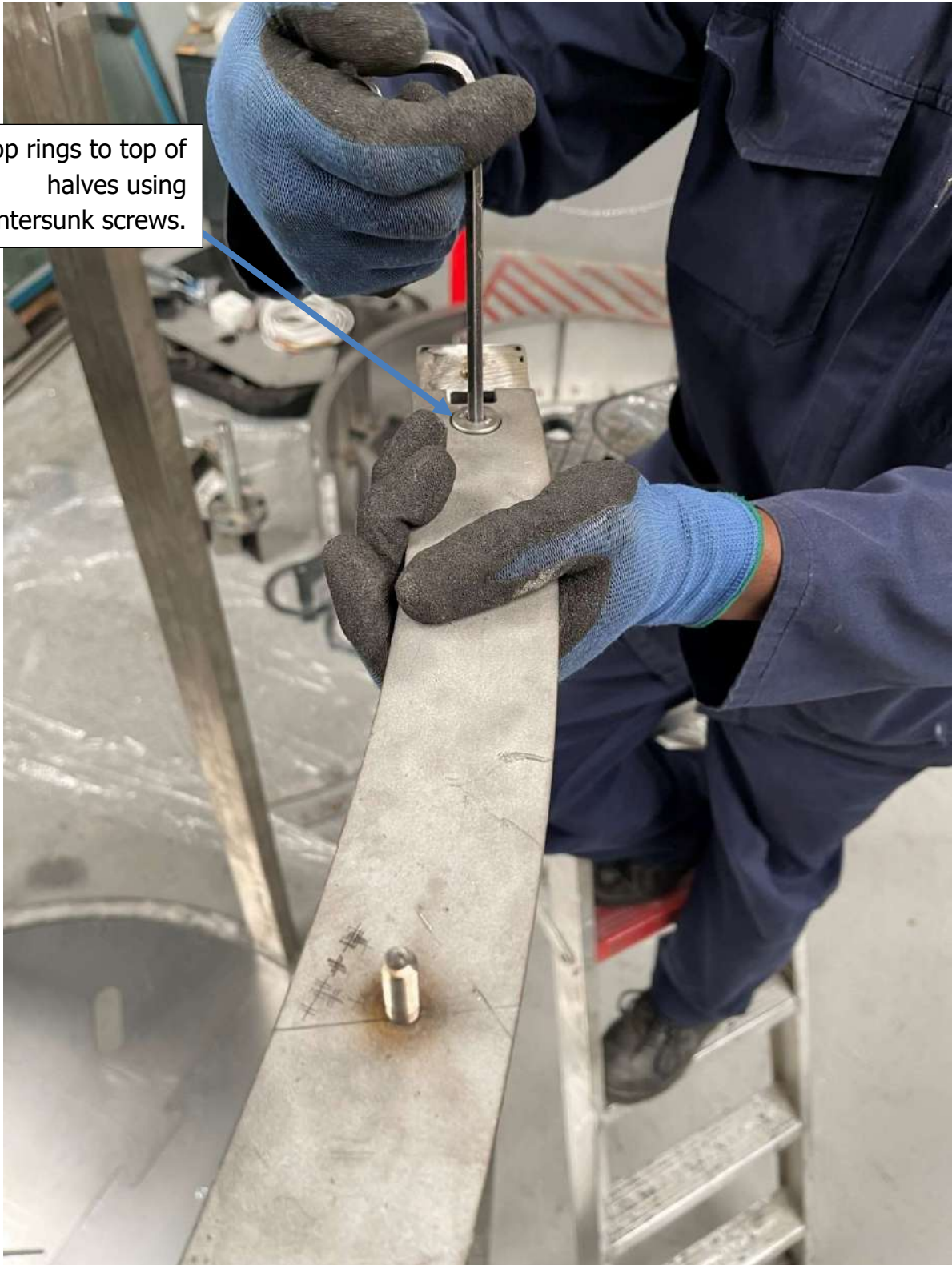
Figure 34: Fitting top ring to side halve
