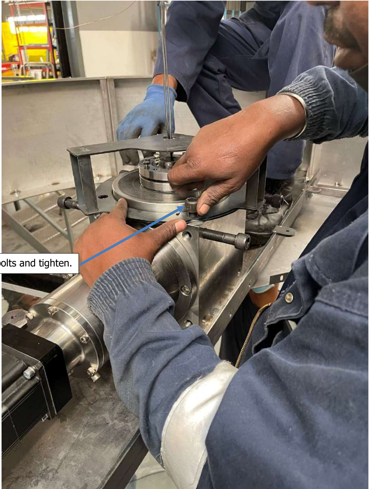
Figure 97: Slip ring structure & proximity plate 2
