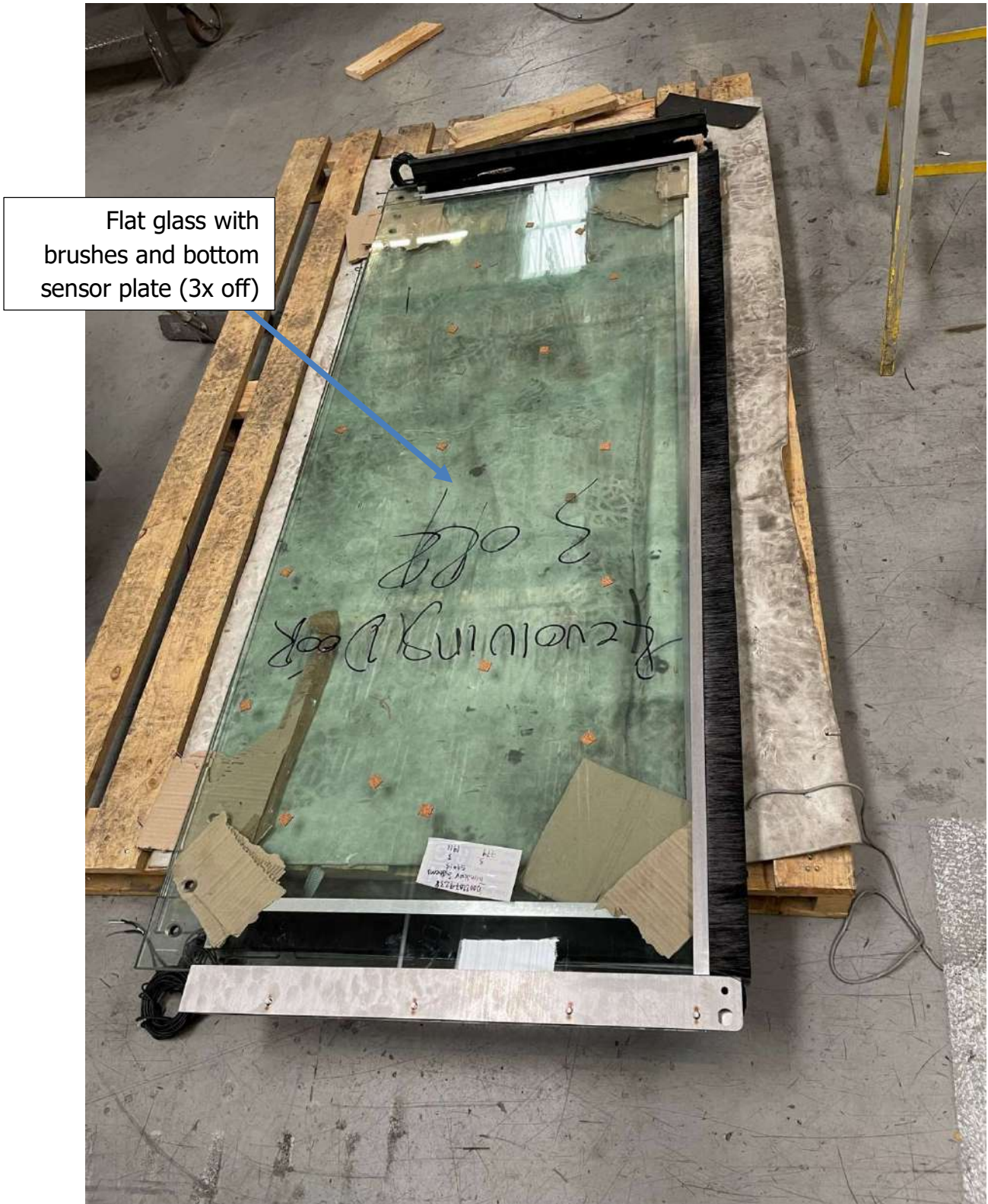
Figure 14: Flat glass, brush and bottom sensor assembly
