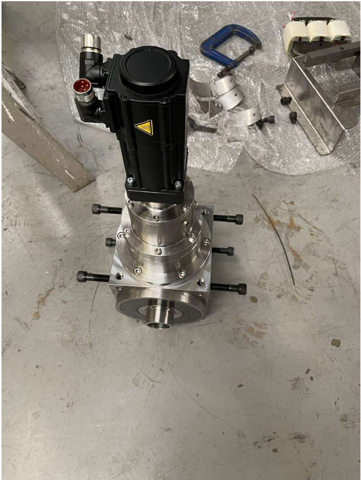
Figure 56: Motor and gearbox
