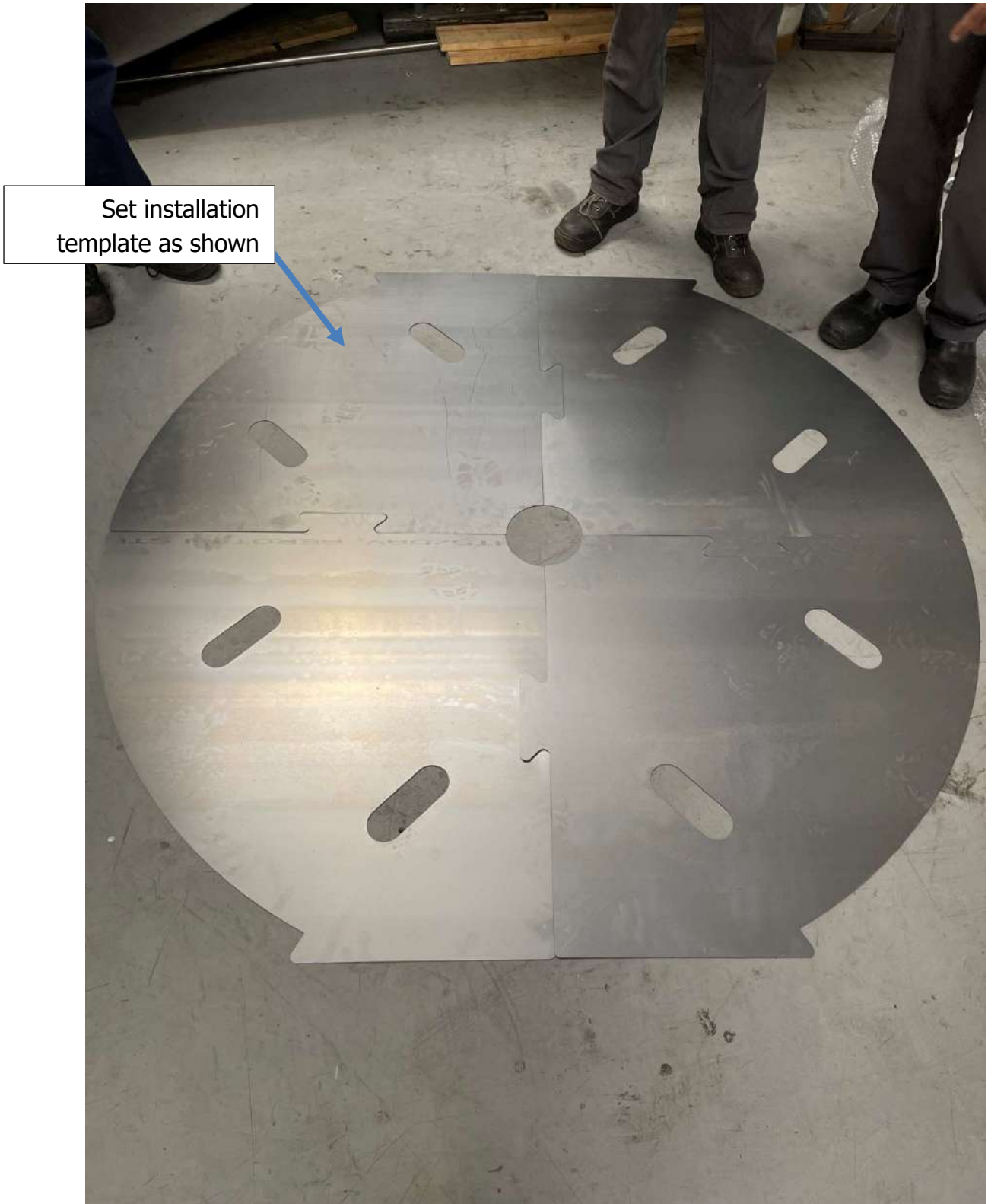
Figure 18: Installation Template placement
