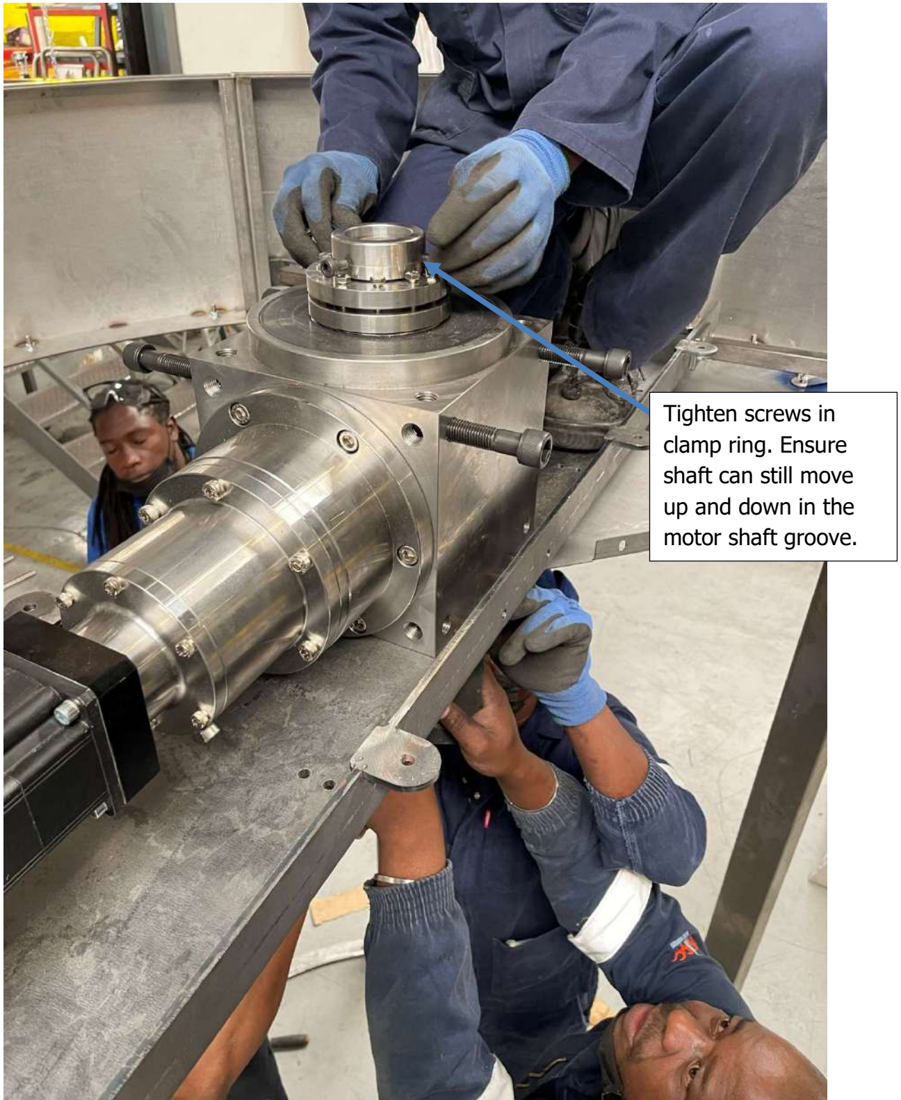
Figure 74: Place and shaft clamp ring 2
