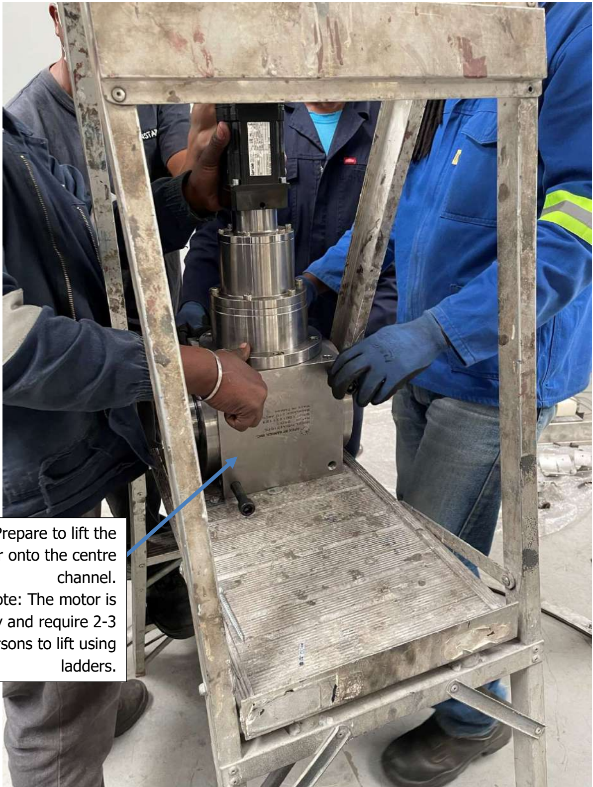
Figure 60: Preparation to lift motor
