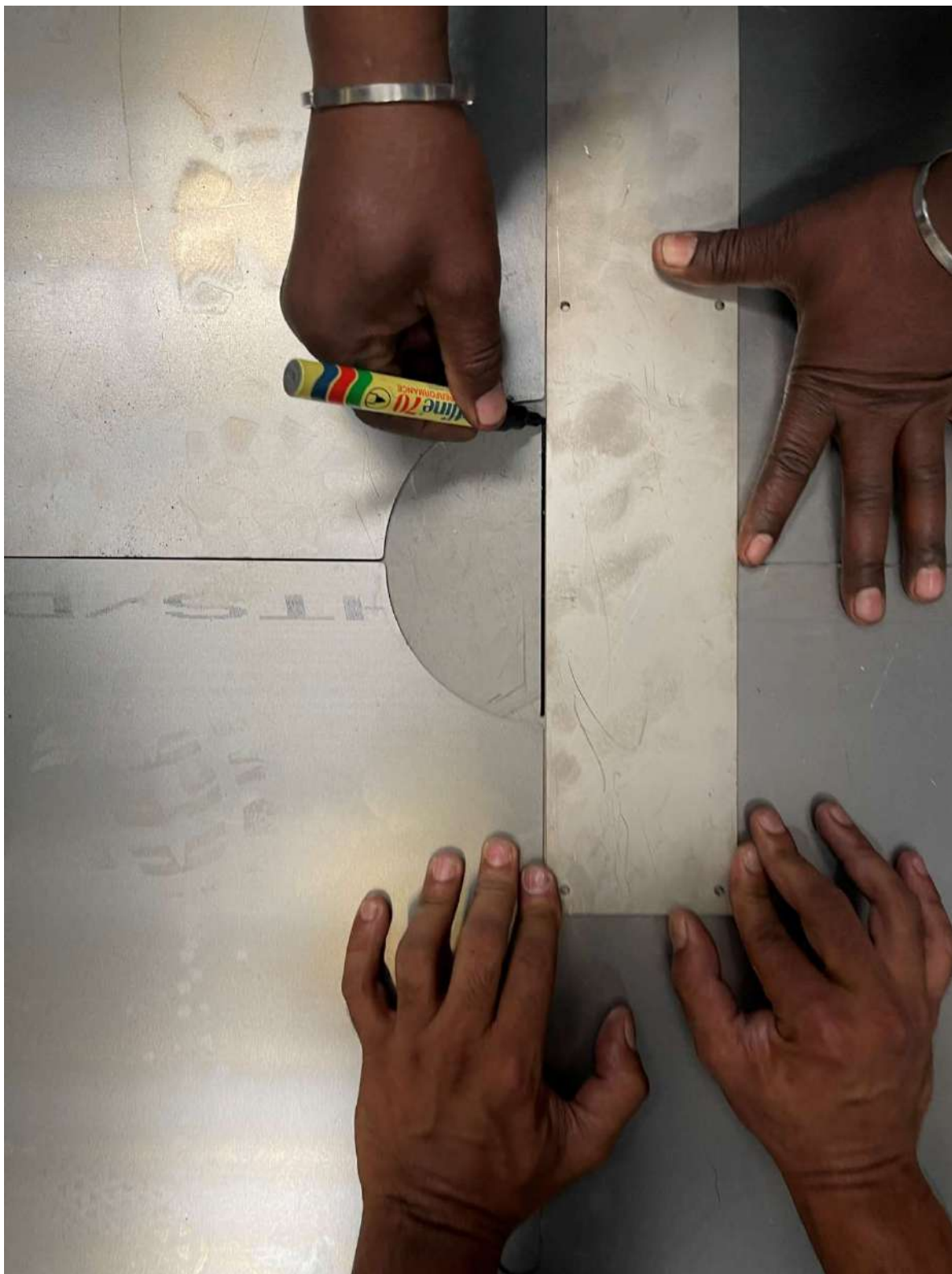
Figure 20: Vertical centerline marked
