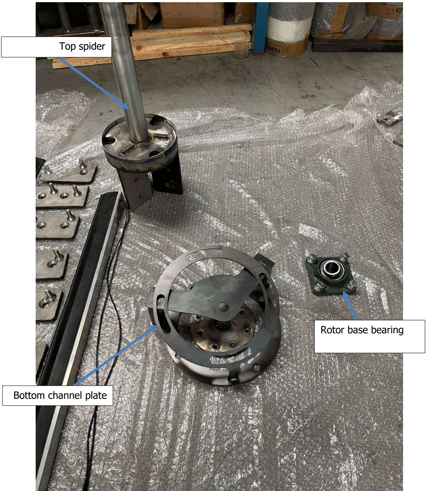
Figure 7: Top spider & bottom channel plate
