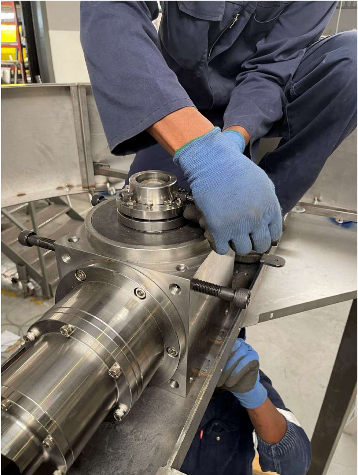
Figure 75: Place and shaft clamp ring 3
