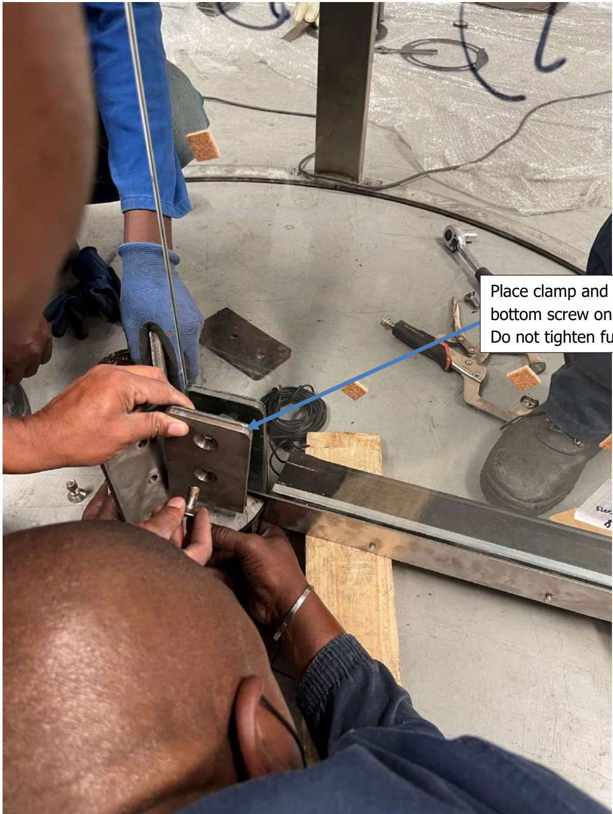
Figure 79: Place glass clamp and screws
