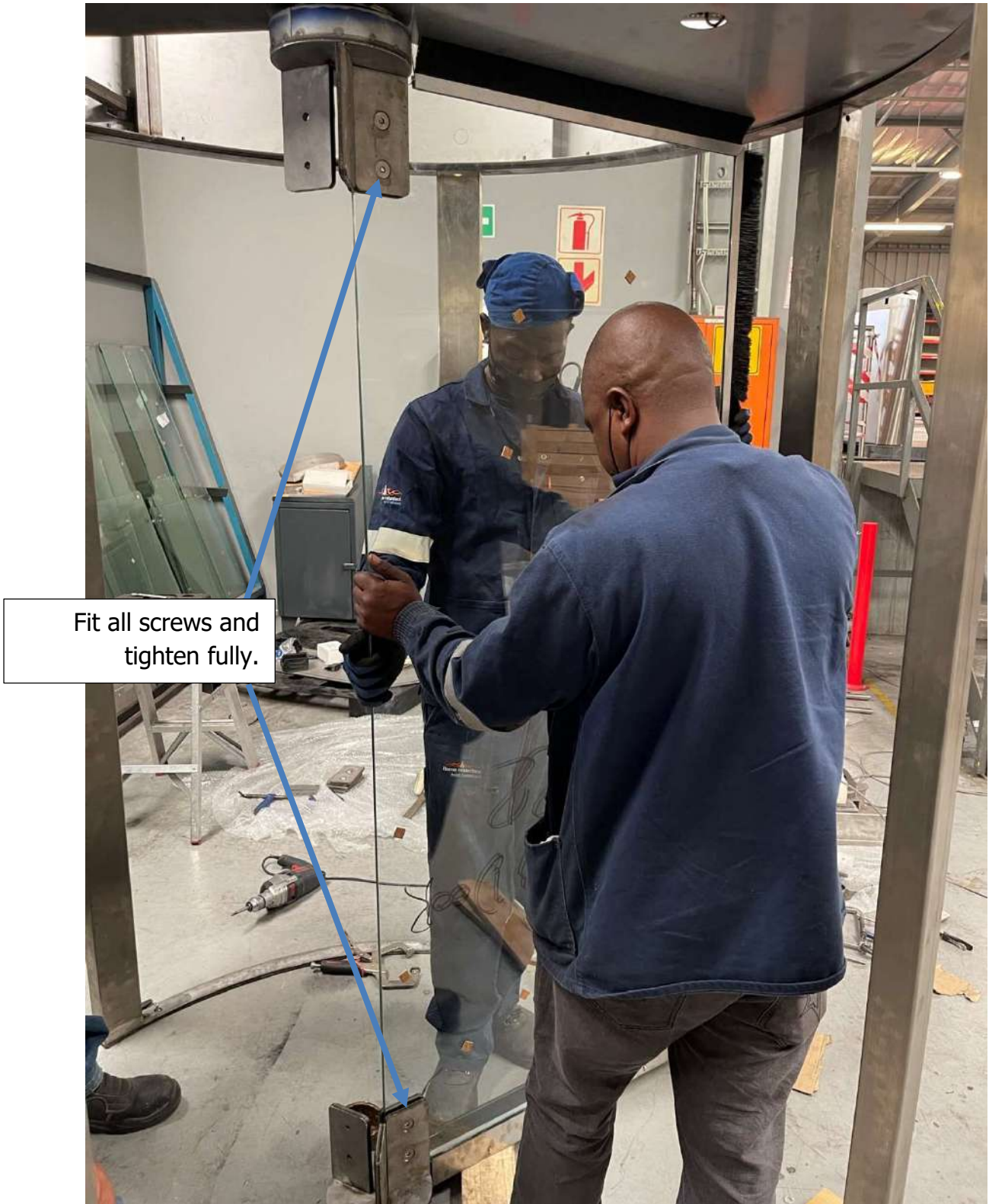
Figure 88: Tighten all glass screws
