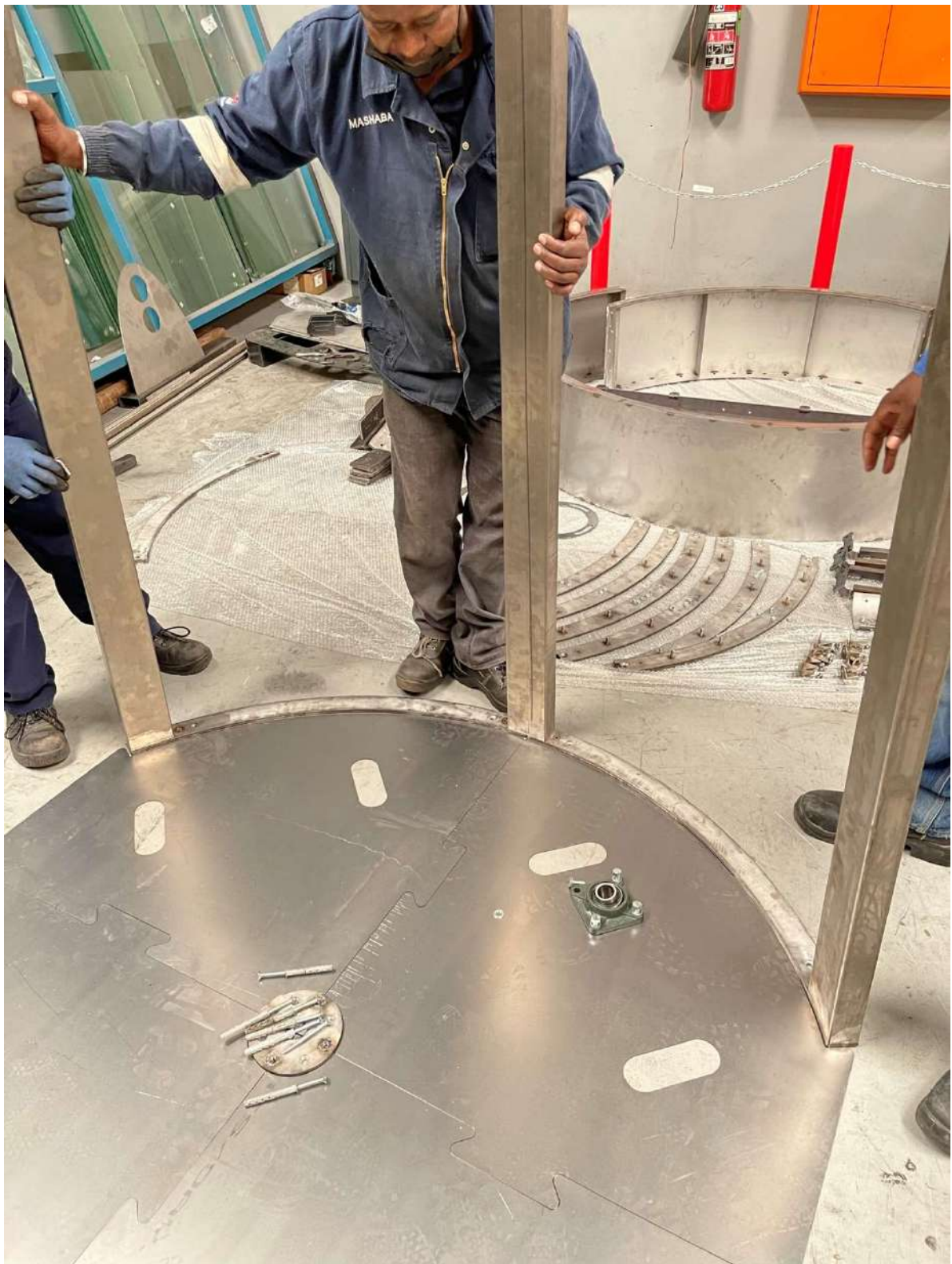
Figure 31: Side half placement on template 2
