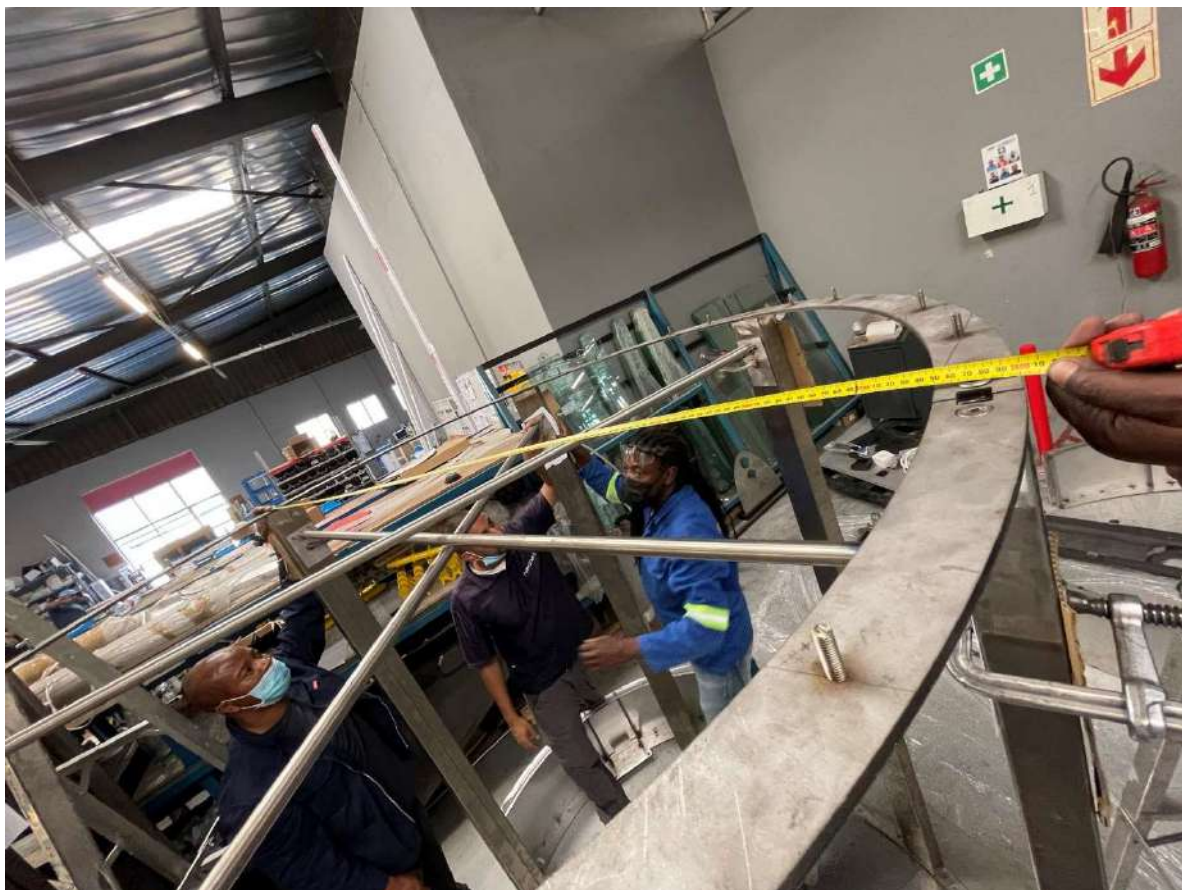
Figure 46: Clamping and measuring between uprights 2
