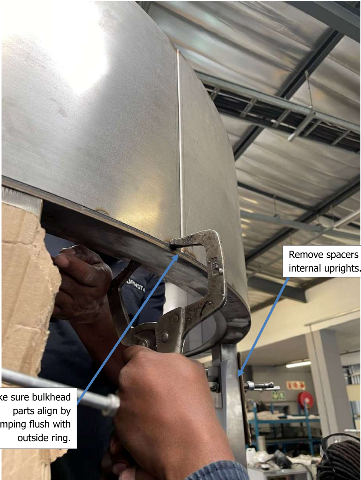
Figure 57: Bulkhead parts check & spacers remove
