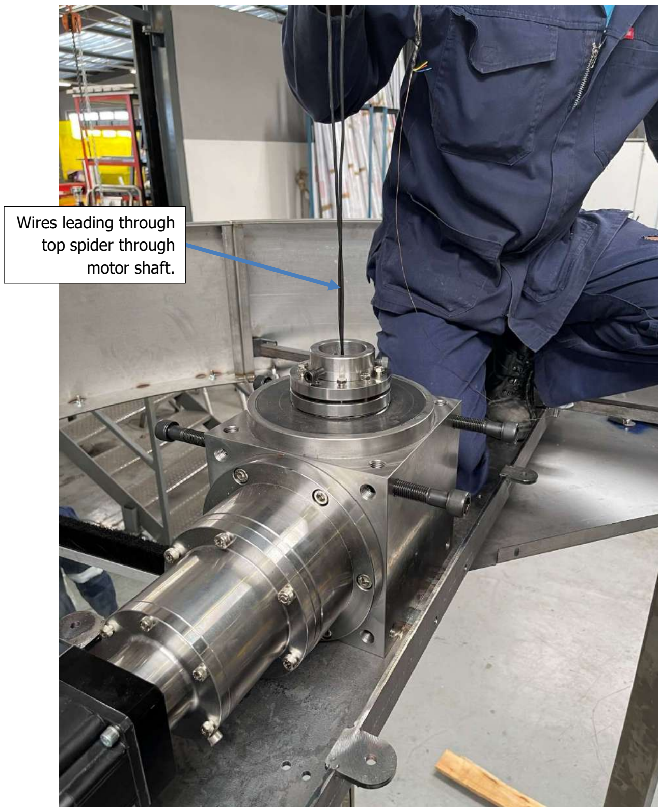
Figure 94: Pull safety sensor cables through motor shaft
