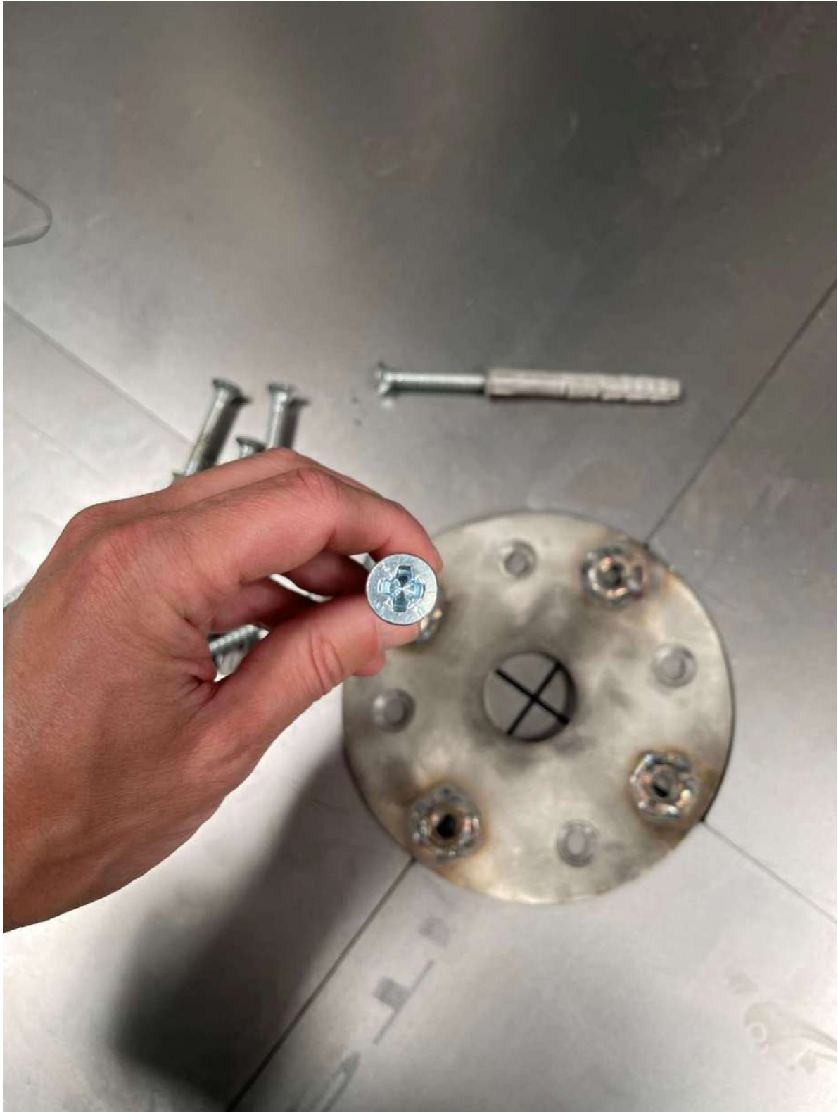
Figure 40: Bearing base ring and anchor screws 2
