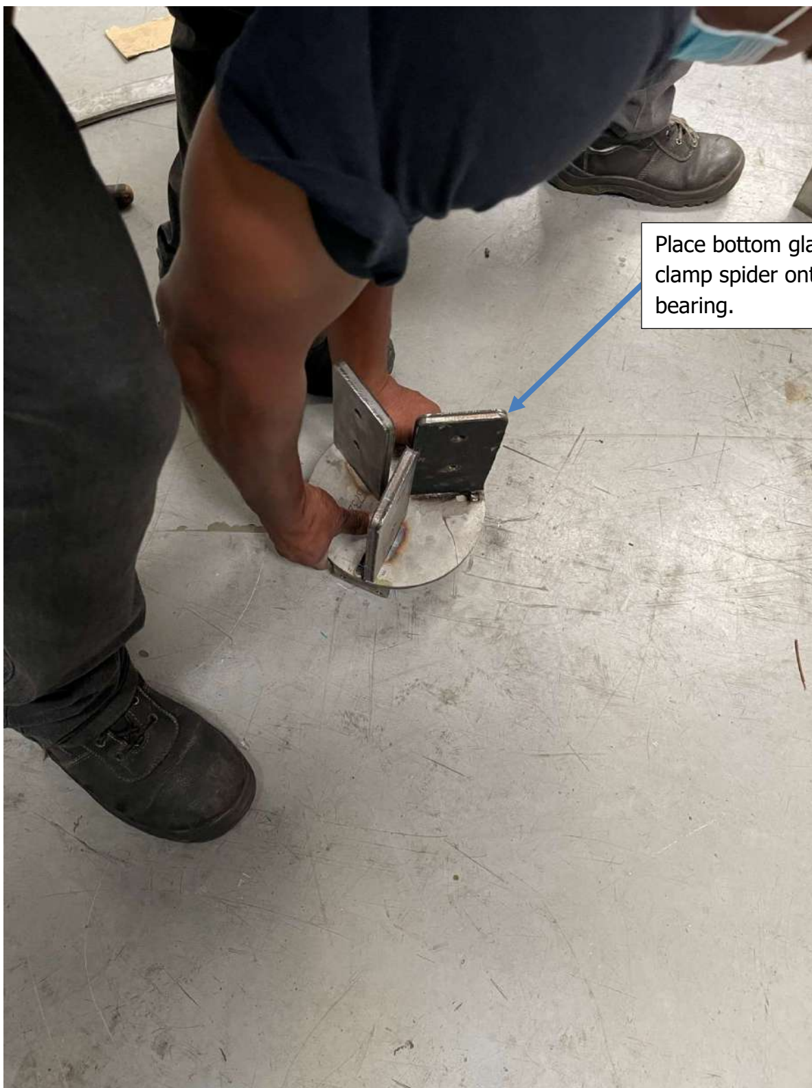
Figure 71: Fit bottom glass clamp spider
