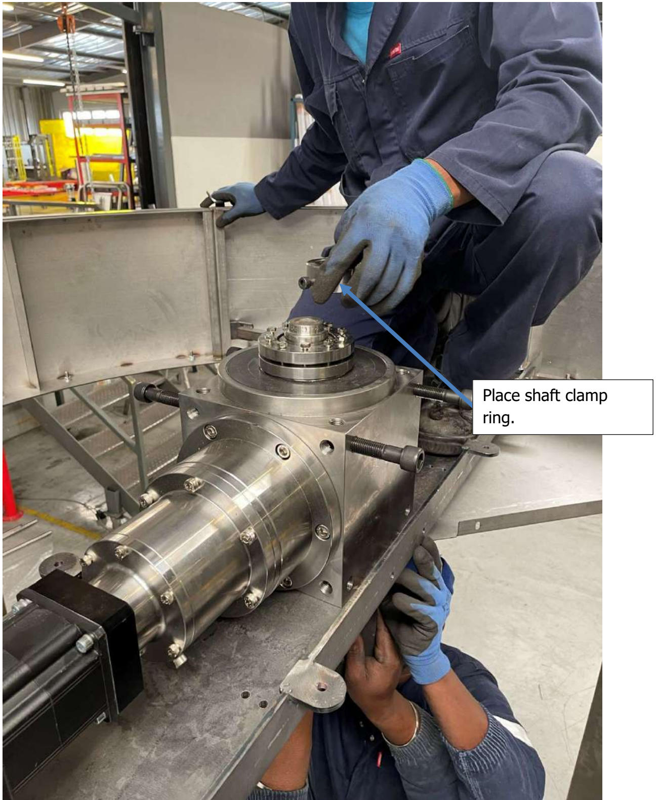
Figure 73: Place and shaft clamp ring
