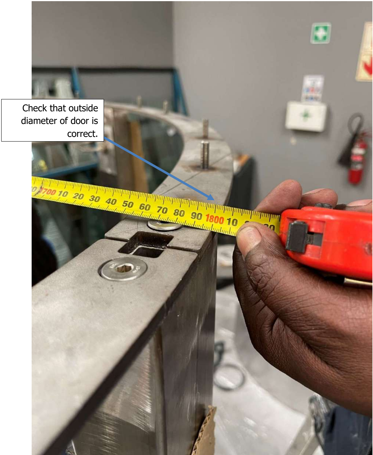
Figure 47: Measuring outside of door
