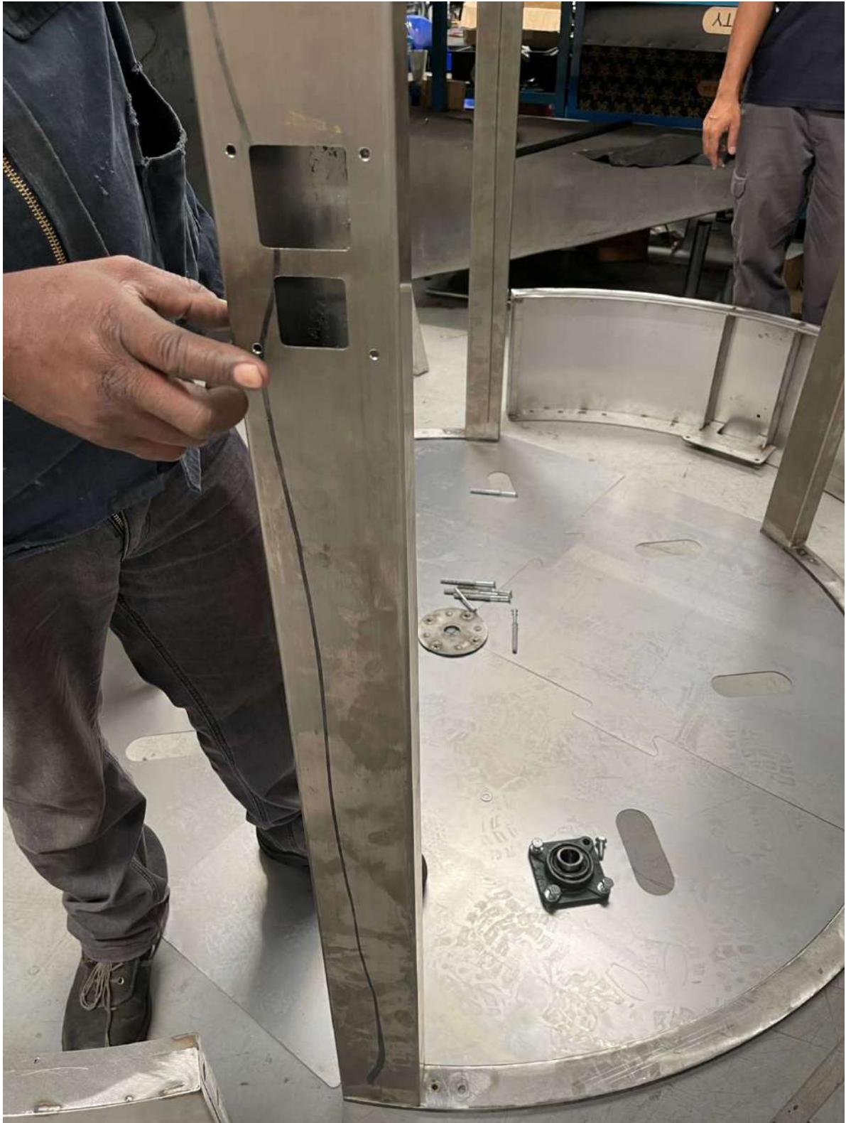
Figure 42: Location of override and stop button on outside upright
