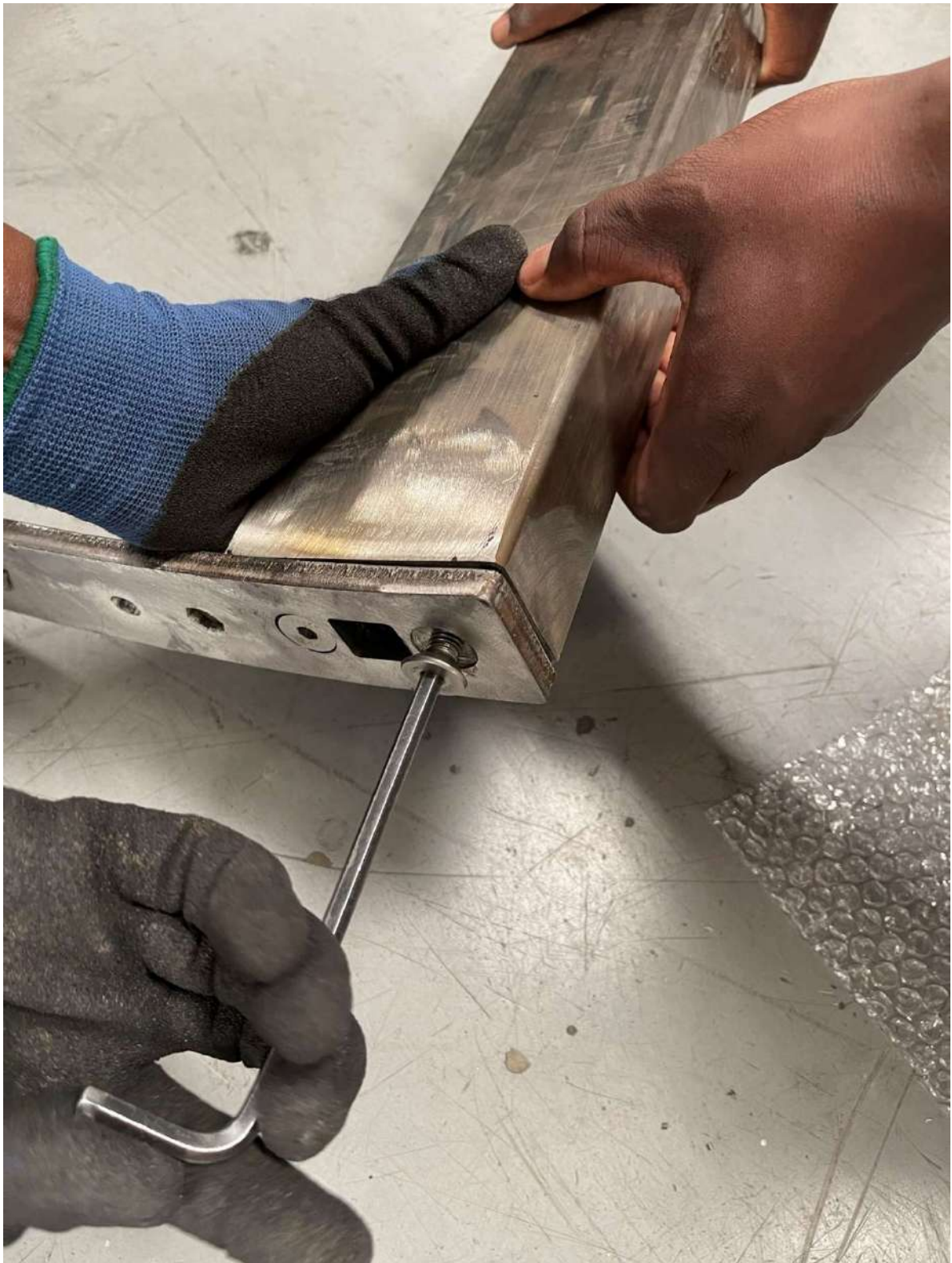
Figure 26: Countersunk screw through bottom ring into upright
