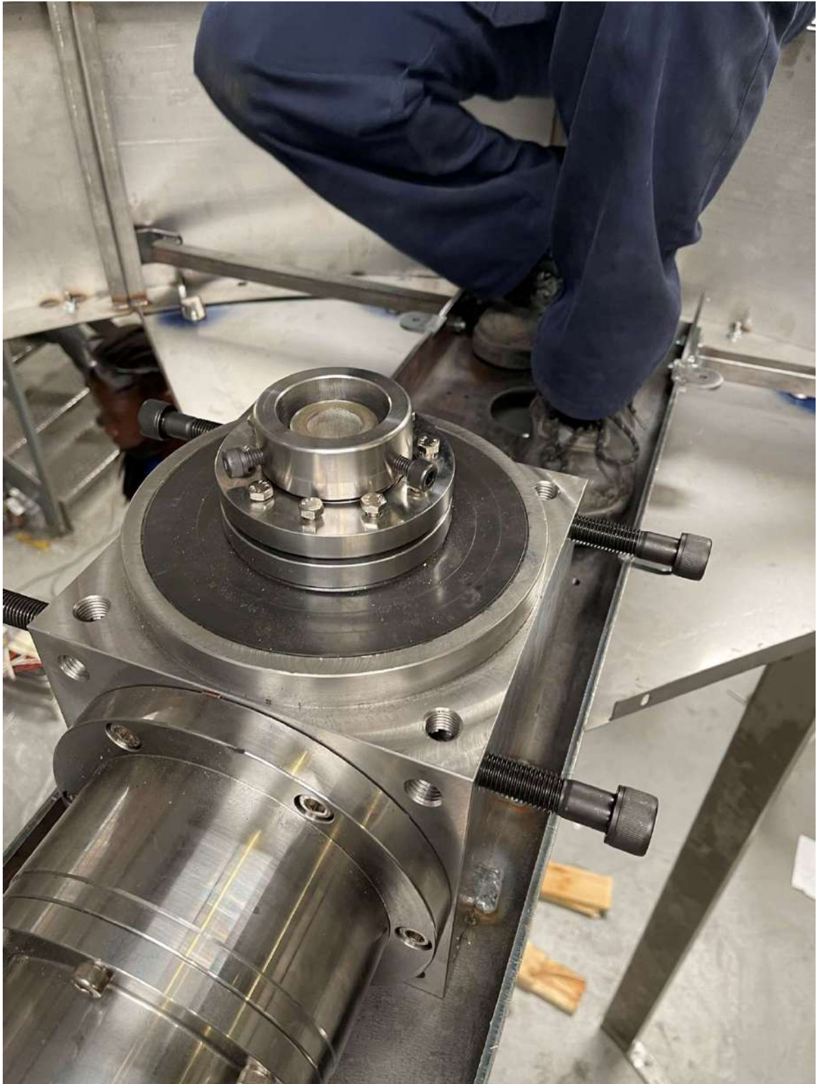
Figure 76: Place and shaft clamp ring 4
