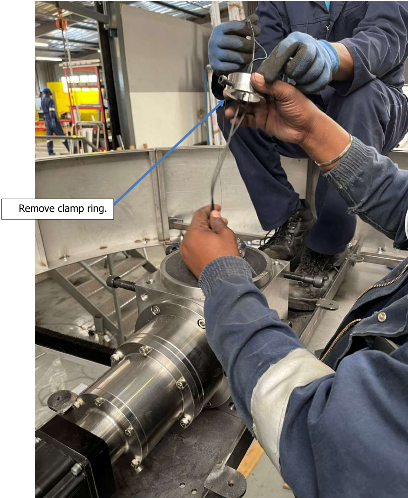
Figure 95: Remove clamp ring
