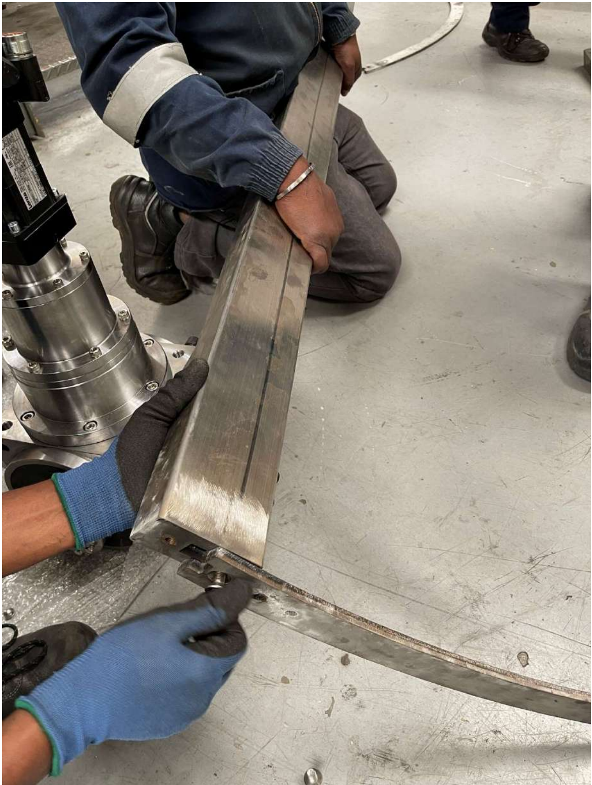
Figure 27: Mid upright bottom ring assembly
