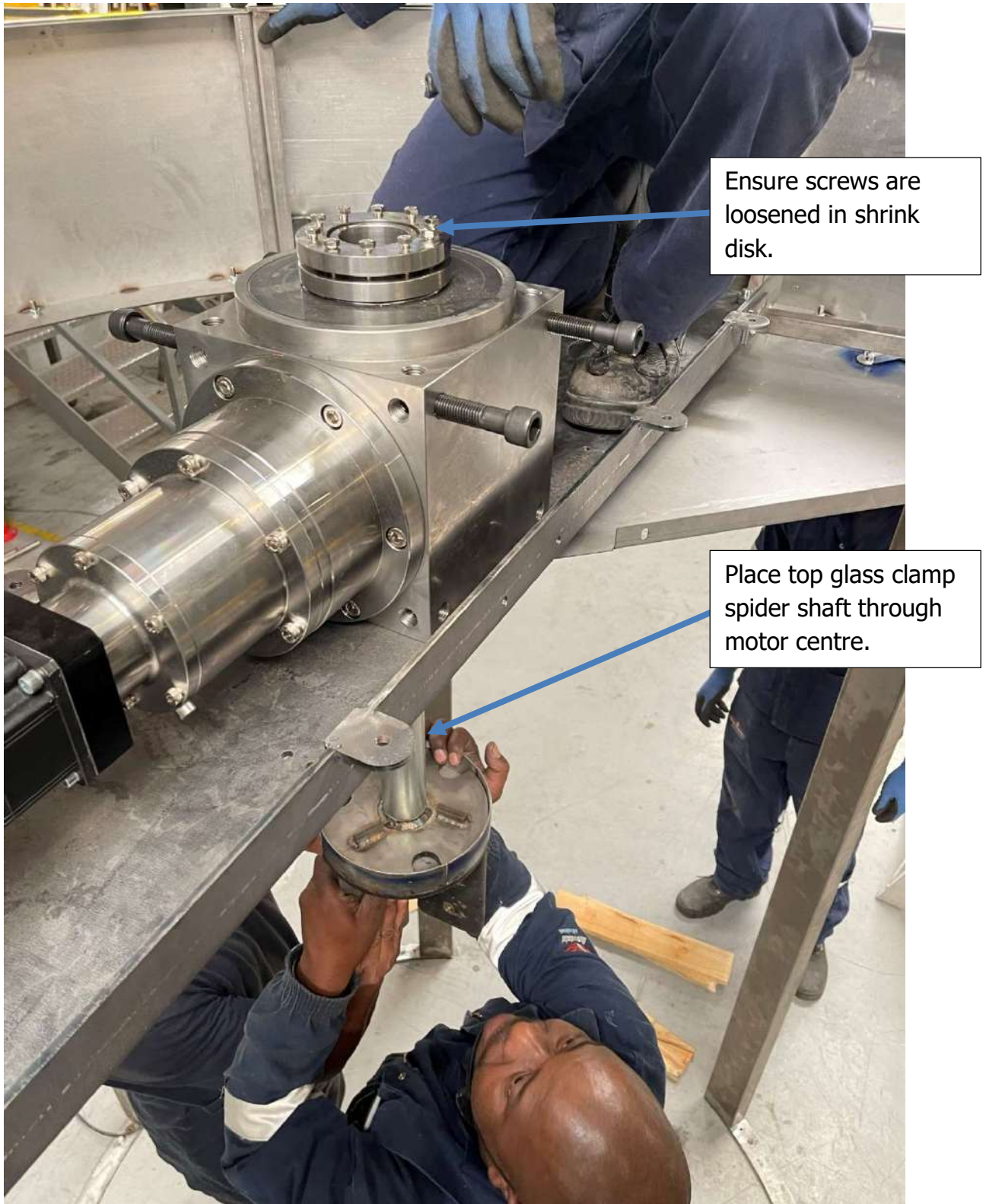
Figure 72: Fit top glass clamp spider
