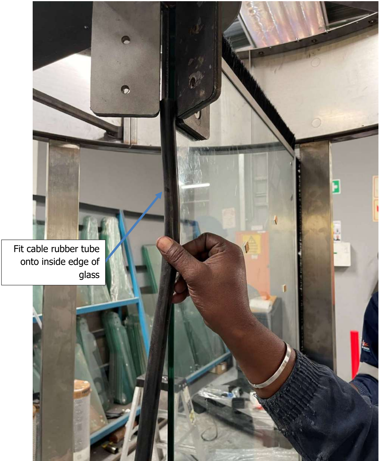
Figure 89: Fit center cable rubber tube
