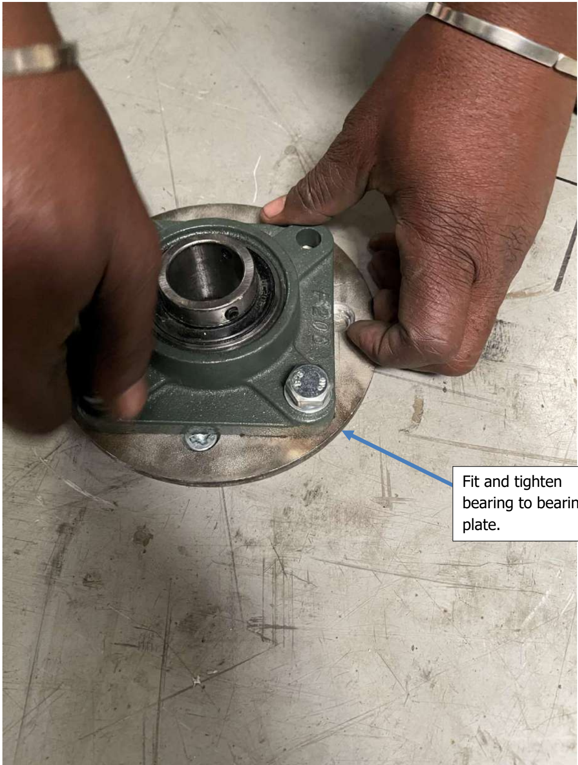
Figure 70: Fit base bearing
