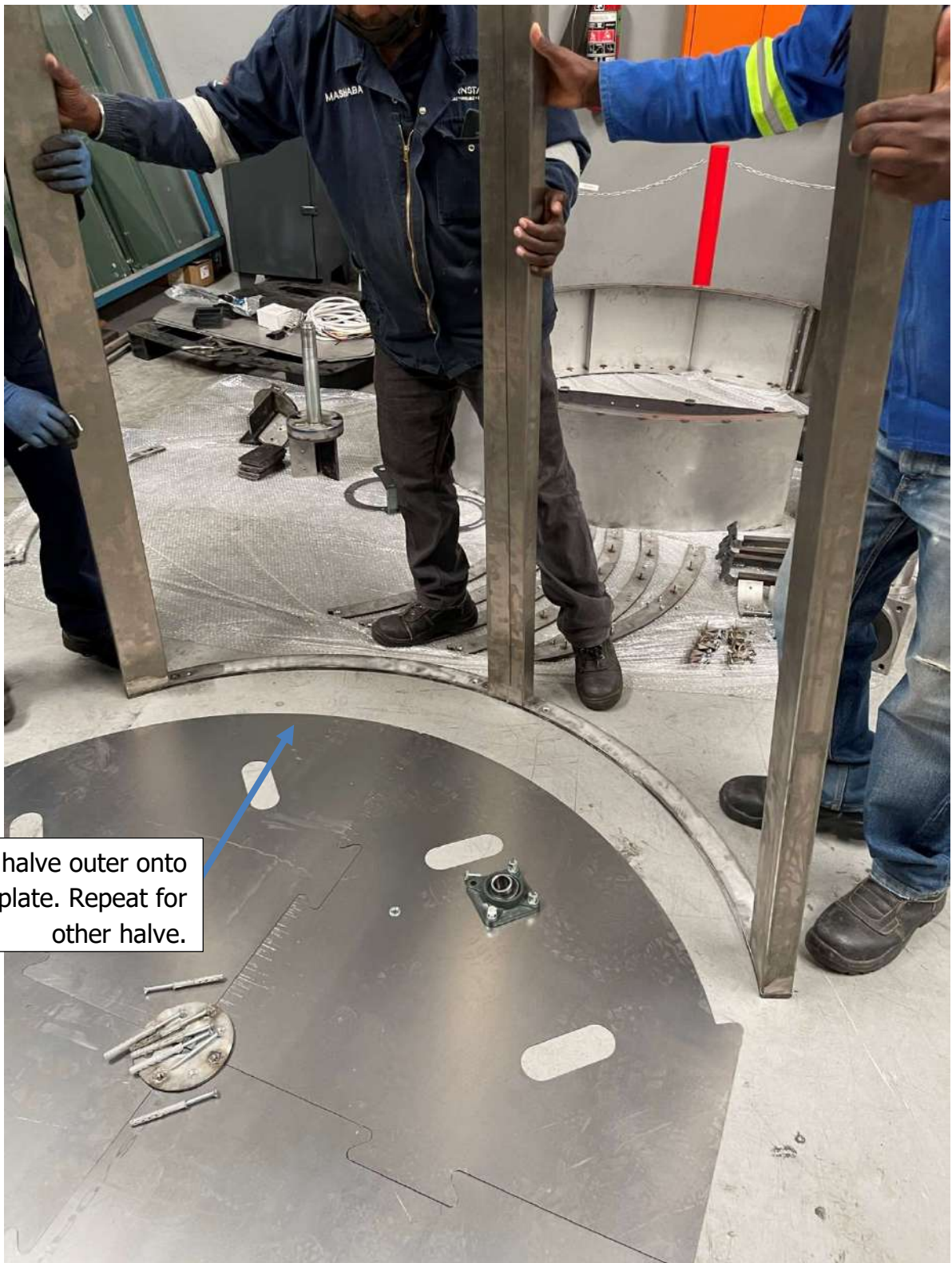
Figure 30: Side halve placement on template
