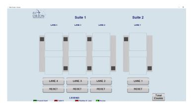
The Orion Entrance Control SpeedLane™ turnstiles are enhanced by incorporating the Infinity Remote Lane Control™ (IRLC) software. The IRLC is a user-friendly lane control software that is intuitive and offers an array of support for end users and integrators.
