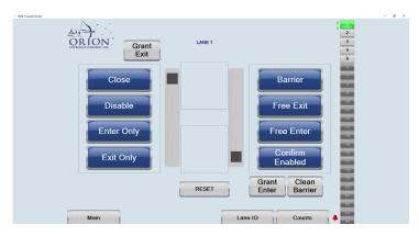
Orion's Infinity Remote Lane Control software offers a robust set of features, including advanced alarm type display, technical service tools, lane beam status, I/O status, and on-the-fly volume adjustment.
