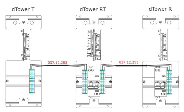
**NOTE** - On the cable itself there are rings identifying where each cable must be connected.
