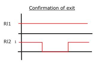
In this operation mode, the output Rl1 can be used to activate an electromechanical counter in order to count the passage flow in the direction of entry of the equipment. Similarly, the output Rl2 can be used to count the passage flow in the direction of exit.
