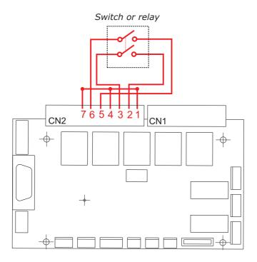
**NOTE** - Switch or relay with two poles and one activation
