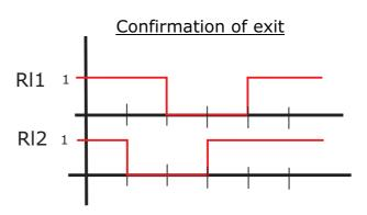
In this operation mode, any of the passage confirmation outputs – output RI1 or RI2 – can be used to activate an electromechanical counter in order to count the passage flow in both directions of the equipment.
