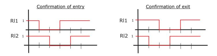
In this operation mode, any of the passage confirmation outputs – output Rl1 or Rl2 – can be used to activate an electromechanical counter in order to count the passage flow in both directions of the equipment.
