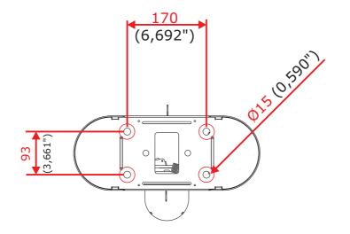
**NOTE** - Measurements are illustrated in millimeters and (inches).
