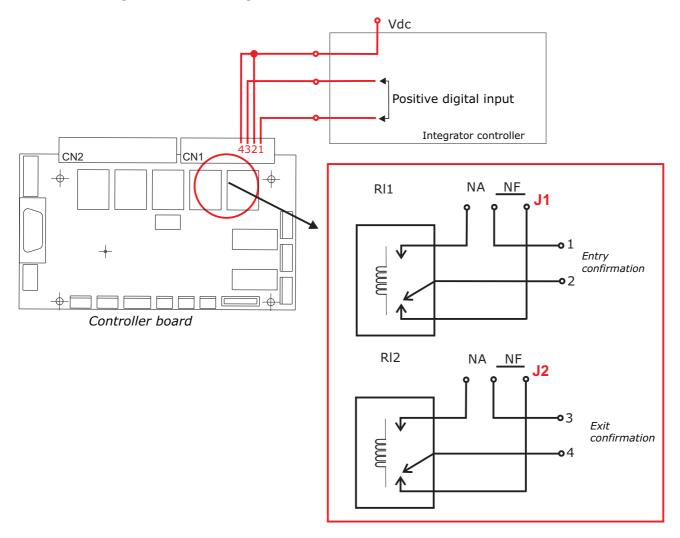
Vdc - True logical level, configured in "disk emulation" DIP Ds2 n.7 in ON.
