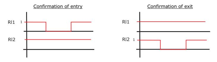
In this operation mode, the output Rl1 can be used to activate an electromechanical counter in order to count the passage flow in the direction of entry of the equipment. Similarly, the output Rl2 can be used to count the passage flow in the direction of exit.
