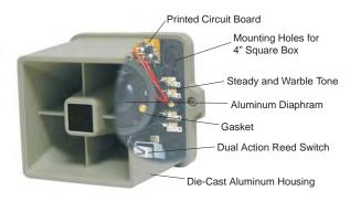
The Small Footprint Siren and Strobe Alarm is an indoor/outdoor, self-contained, 15 watt, armored security siren. The full featured siren consists of a single tone that delivers a warble sound output, light weight, rust-proof aluminum die-cast housing, a 122 dB output siren driver, and a dual action normally open reed plunger switch for normally closed loop. The armored siren does not require additional modules, metal boxes, tamper switches, special tools, or training to install and operate.
