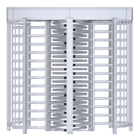
Extremely robust and water resistant, 3 section full height turnstiles in stainless steel; hot-dipped galvanized or galvanized plus powder coated finish. Bi-directional, logic controlled. Hand operated and motor driven with electro-magnetic lock options available.
