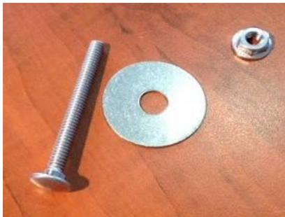
Use for bolting **side walls to fiberglass angle**. 1/4-20 x 2-1/2" carriage bolt, 5/16" ID x 1-1/2" OD washer and 1/4-20 serrated flange nut.
