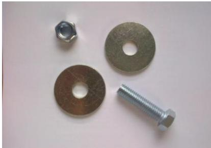
Use for bolting **side wall panel** internal flanges together. 1/2-13x2" hex cap bolt, 1/2" ID x 2" OD washer(2) and 1/2-13 hex nut.
