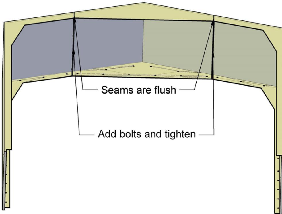
Once the side panel is lined up with the roof panel, clamp it into place and install a ½"-13 x 2" hex cap bolt assembly through each of the pre-drilled holes between the two parts.
