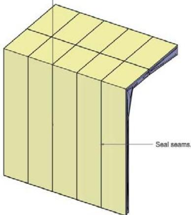
Panel Assembly: Caulking and Sealant: Roof Only:
