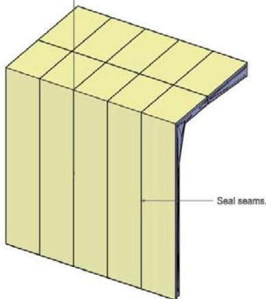
Panel Assembly: Caulking and Sealant: Roof Only:
