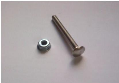
Use for bolting **end panels to side walls**. 1/4-20 x 1-1/2" carriage bolt and 1/4-20 serrated flange nut.
