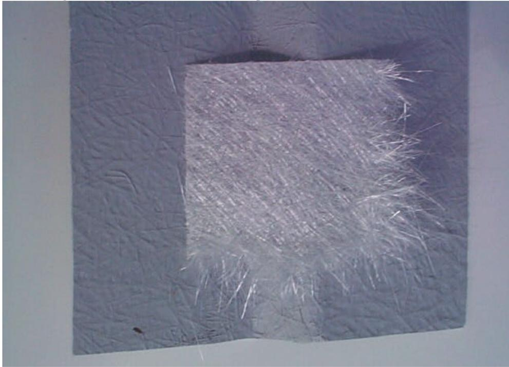
**Step 4:** Mix the resin required with catalyst also supplied in the repair kit. Ratio of 1 quart of resin to 1 – 1 ½bsp of catalyst. Wet the glass cloth with resin and apply to the hole or crack on the inside surface. Using a brush work out the air bubble to ensure good surface contact.
