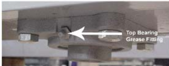
Figure 4.4 – Lubricating the bottom bearing of the top channel
