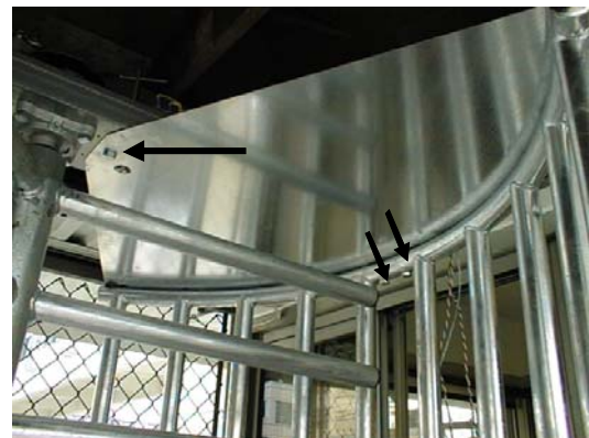
Figure 3.21 - The bolt locations to mount the yoke section to the top channel are identified with white arrows. The bolt location to mount the yoke guard plate to the top channel is identified with a black arrow.
