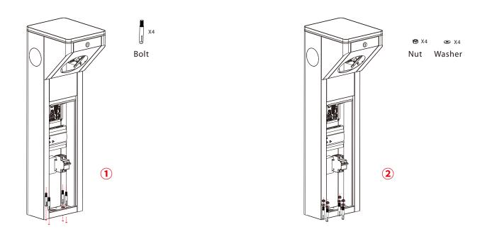
**Note:** Before inserting the bolt, the user must pull the power cable and Ethernet from the machines and put them into the wire slot.
