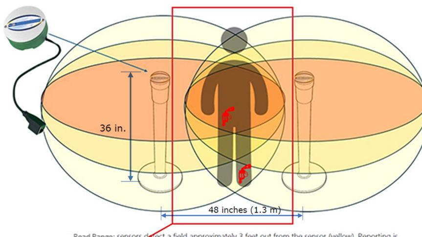
Read Range: sensors detect a field approximately 3 feet out from the sensor (yellow). Reporting is focused on the overlapped region that is common for both sensors (middle). Red is most sensitive area of detection.
