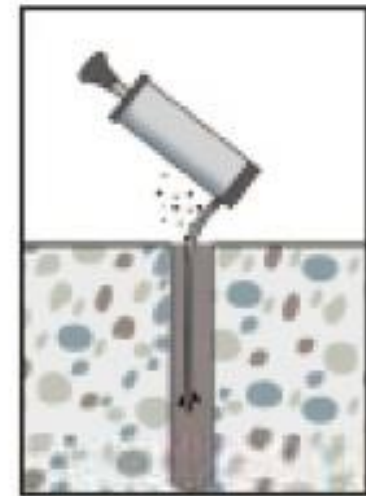
2. Clean hole (blowing)
