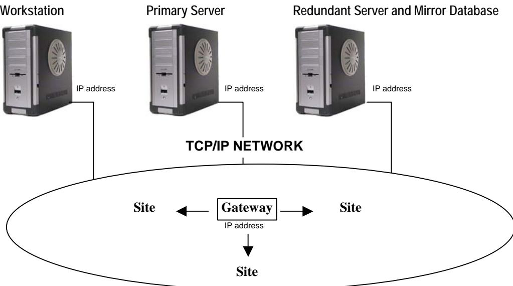
The Redundant Server monitors the communication between itself and the Primary Server. The Mirror Database is a real-time copy of the system database and Windows system registry entries.
