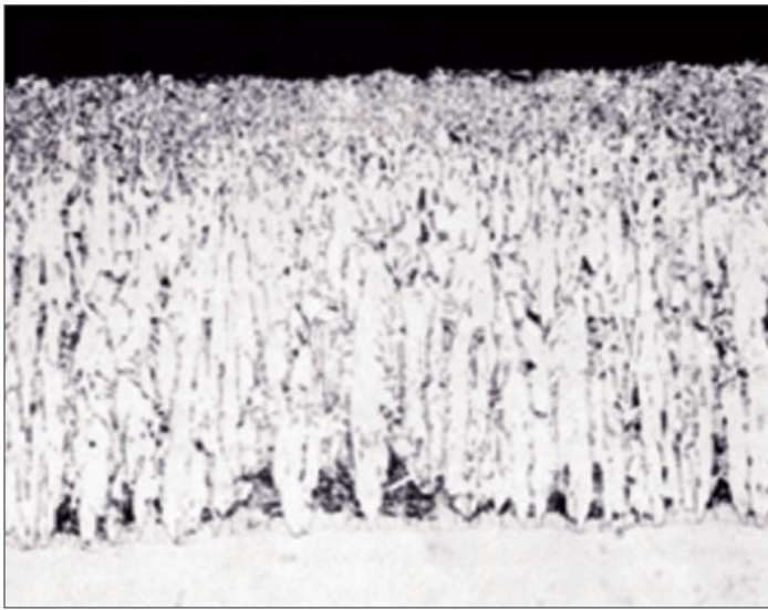
Figure 7: Irregular zinc alloy layers
