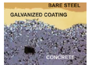
Figure 16: Elemental map of galvanized rebar. The corrosion products of galvanized rebar are less dense and do not build up pressure to cause concrete spalling (unlike the dense corrosion products of bare steel). The zinc corrosion products (depicted right, in white), migrate away from the galvanized coating and disperse into the concrete matrix.
